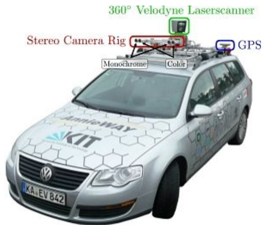
Figure 9. Sensor car used to record information for the KITTI dataset [25].
